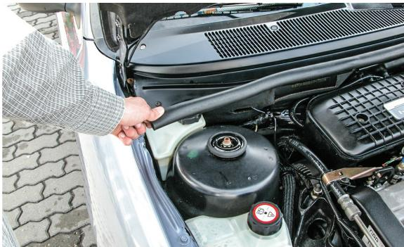
(EN) Remove the rubber seal
