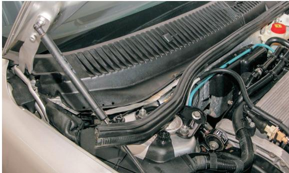
(EN) Remove the rubber seal
