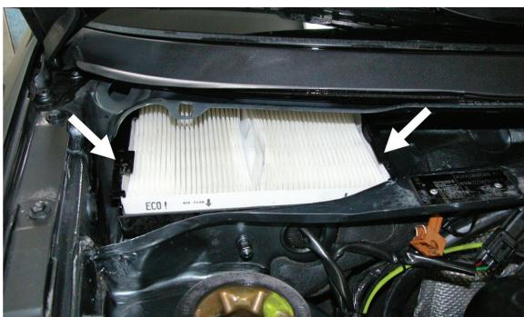
(EN) Unlatch the filter from its socket
