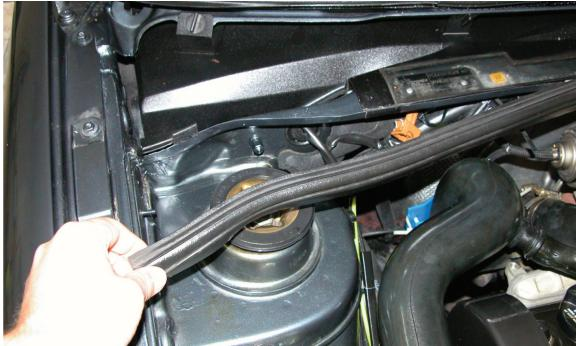
(EN) Remove the rubber seal
