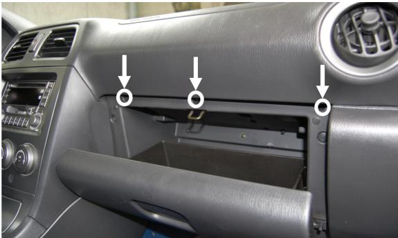
(EN) Remove the glove compartment
