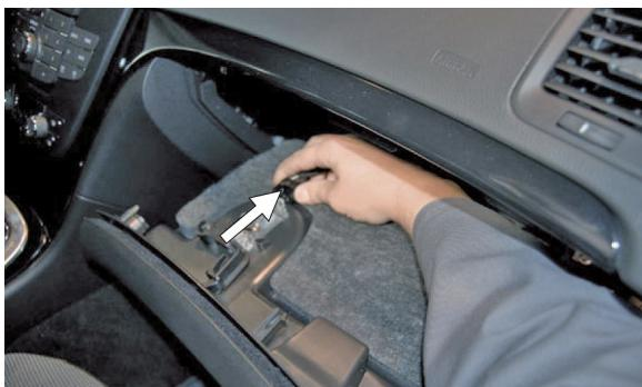
**(EN)** Disconnect the electric circuit
