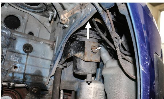
(EN) Loosen clamping ring fastening the filter, take filter out
