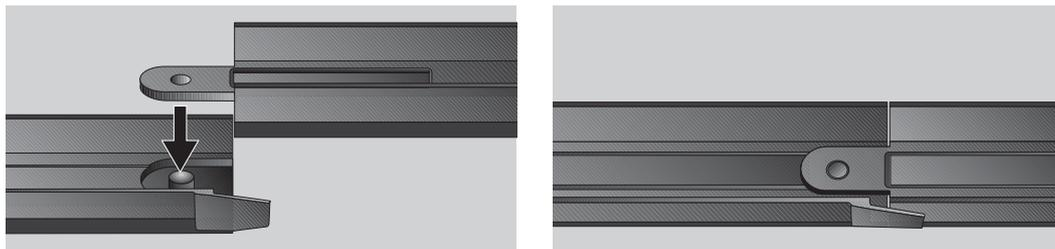
Push the base into the groove at the marked points.
