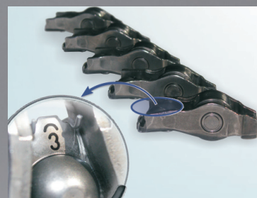
Image 2: Rolling contact rocker arm marking
