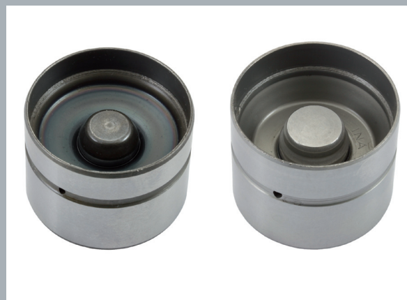
Figure 2: Hydraulic bucket tappet, left: old version, right: new version
