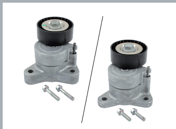
Image 1: Tensioning arm 56653 – Left, old version with fixing screws. Right, new version with fixing screws.
