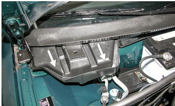
**EN** Remove the filter housing
