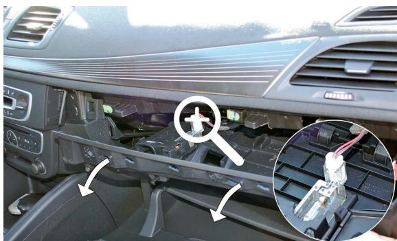
(EN) Disconnect the electric circuit. Remove the locker
