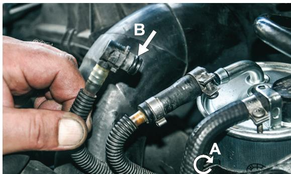
**EN** Tighten clamping ring fastening the filter (A), fix a new gasket on the fuel outlet connection
