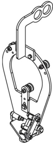
Fig. 1: Assembly aid with transport handle cDISK Blitz Rotary item-no. 3745410
