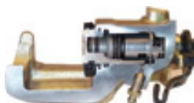
1.1 In some Bosch types left and right threads for adjustment of piston can occur.
