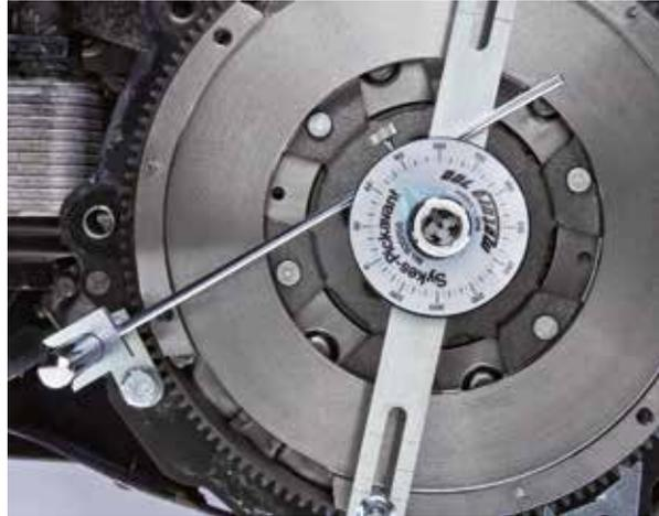
7. Use the slotted arm to rotate the secondary mass anticlockwise until the arc spring force can be felt.
