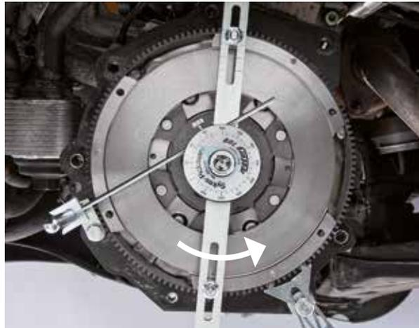
8. Slowly release the slotted arm, allowing the arc springs to relax. Set the degree gauge pointer to "0".
