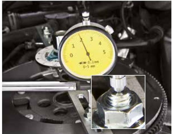
3. Gently push the slotted arm towards the engine (using your thumb, for example) until resistance can be felt.
