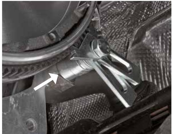
5. Use the slotted arm to rotate the secondary mass anticlockwise until the arc spring force can be felt.
