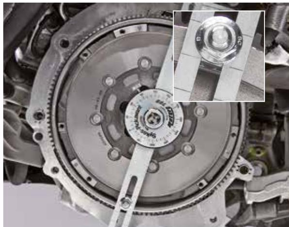
4. Lock the DMF using the locking dogs and, if necessary, appropriate spacers to align the locking tool flush with the starter ring gear.
