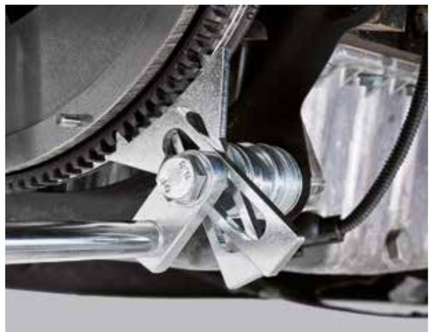
6. Fit the degree gauge locking bar to the degree gauge and the dial gauge stand and tighten the knurled screw.
