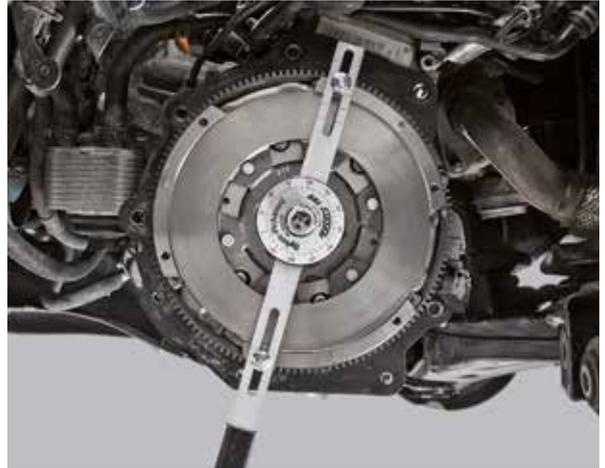
There are a few DMF types with an odd number of threaded holes for the clutch pressure plate, making it impossible to mount the slotted bar centrally. In this case, the freeplay angle must be measured by counting the teeth of the starter ring gear – see Chapter 7.3.
