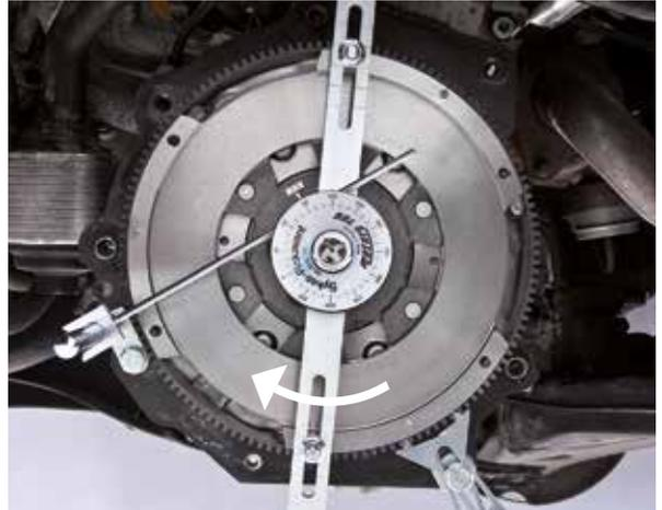
10. Slowly release the slotted arm, allowing the arc springs to relax. Read off the degree gauge and compare the measurement against the rated value – see rated value table in Chapter 8.
