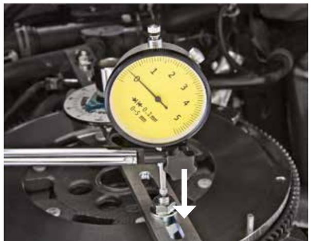
4. Pull the lever gently in the opposite direction (using your finger, for example) until resistance can be felt. Read off the dial gauge and compare the measurement against the relevant rated value – see rated value table in Chapter 8.
